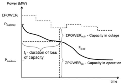
Fig. 3. Graphical representation of parameters for determining improved loss of load expectation
