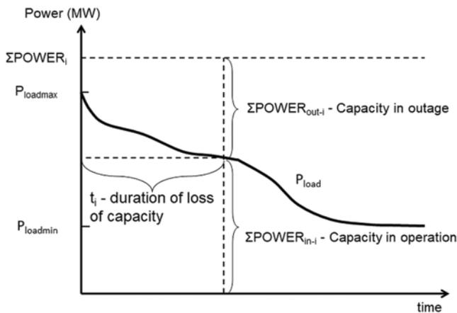
Fig. 1. Graphical representation for determining the loss of load expectation
