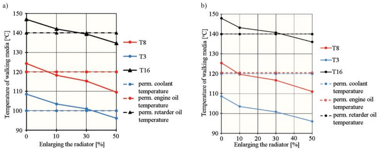
Fig. 10. Temperature of cooling media  $T_8$ ,  $T_3$ ,  $T_{16}$  versus coolant flow  $T_{ot}$  (simulation): (a) for water, (b) for glycol
