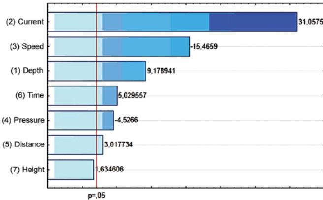
Fig. 3. The influence of test parameters on the stroke of the cutting traces, q.v. the results of calculations and the Pareto diagram.
