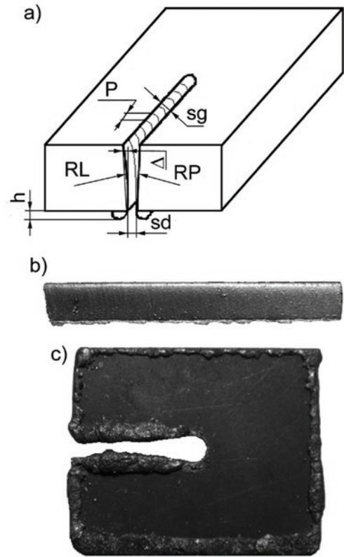
Fig. 2. Sample after plasma-cutting: a) schematic diagram of the test factors, b) lateral surface of the slit, c) lower surface of the sample
