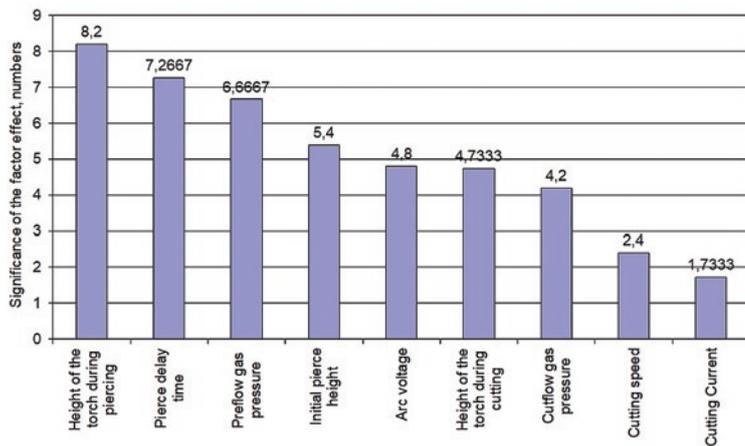
Fig. 4. The significance of parameters in the plasma cutting process according to the expert opinion method
