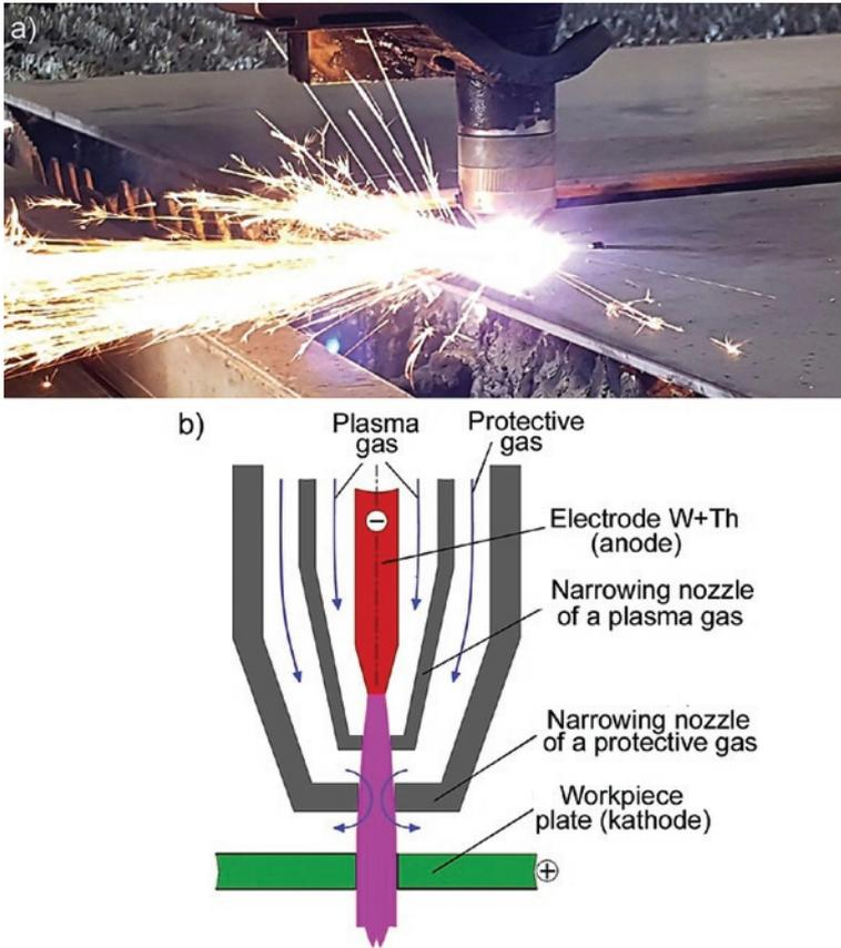
Fig. 1. Plasma cutting (a) and schematic of plasma torch (b)
