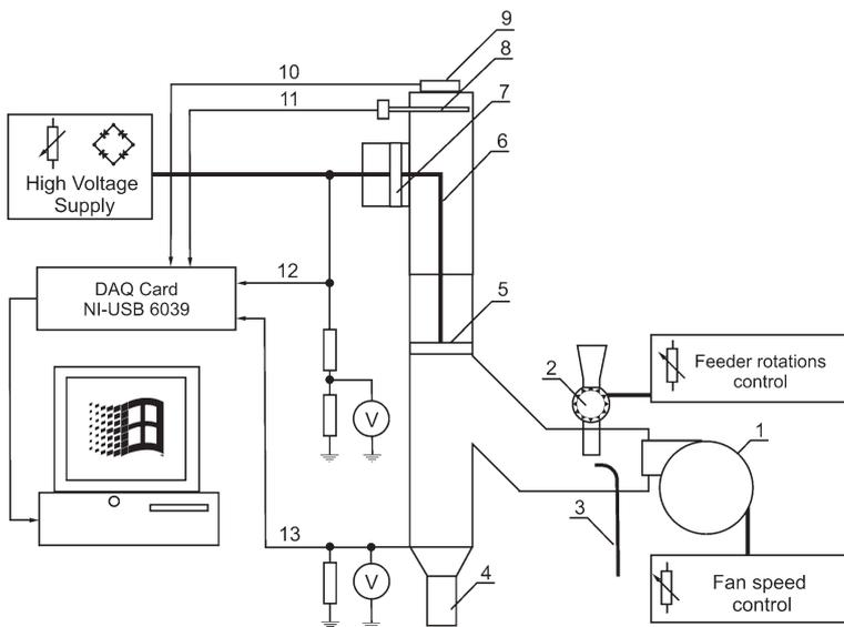
Fig. 2. Simplified diagram of the laboratory ESP 1 - fan, 2 - dust feeder, 3 - compressed air nozzle, 4 - separated dust container, 5 - lower discharge electrode holder, 6 - discharge electrode, 7 - upper discharge electrode holder, 8 - dust meter sensor, 9 - air flow velocity sensor, 10 - air flow measurement circuit, 11 - dust concentration measurement circuit, 12 - high voltage measurement, 13 - ESP current measurement.
