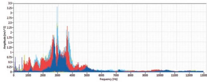
Fig. 2. Frequency spectrum of signals recorded on the milled diameter under load
