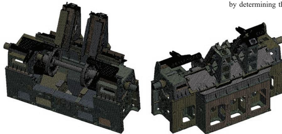
Fig. 4. FEM model of the analysed lathe
