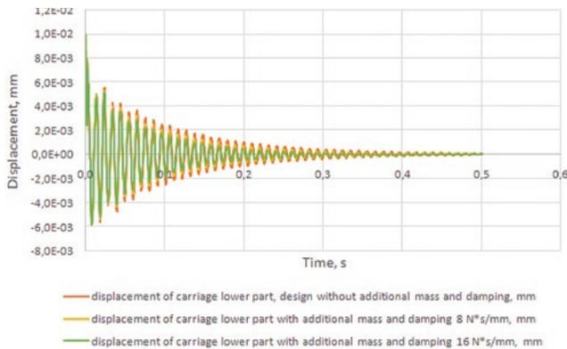
Fig. 10. Displacement of a point in the lower part of the slider to force the harmonic exertion.
