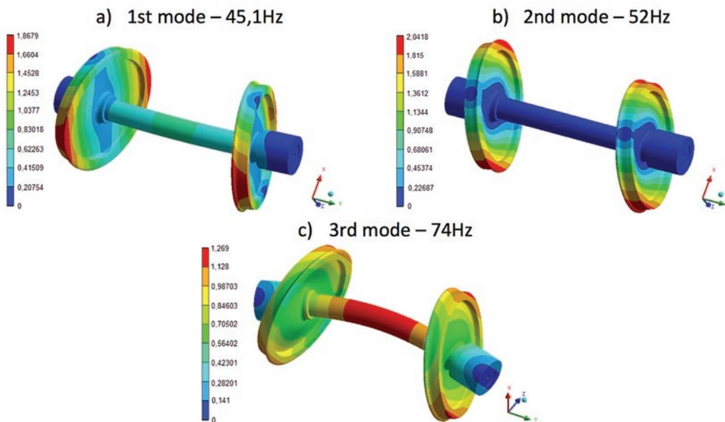
Fig. 5. The first three mode shapes corresponding to the frequencies of the wheelset: a)  $f_1=45,1$  Hz; b)  $f_2=52,0$  Hz; c)  $f_3=74,1$  Hz
