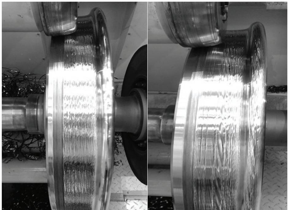
Fig. 1. Comparison of surface finish quality for different machining parameters A)  $A = 5\text{mm}$ ,  $S = 99\text{m/min}$ ,  $f = 1,5\text{ mm/rot}$ ,  $d = 856\text{mm}$  B)  $A = 4\text{mm}$ ,  $S = 90\text{m/min}$ ,  $f = 1,5\text{ mm/rot}$  (21%)  $d = 856\text{mm}$ .
