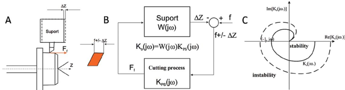
Fig. 11. Self-excited vibrations diagram. A) B) Self-excited vibrations system C) Frequency response to stability loss
