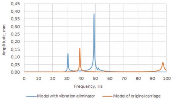
Fig. 9. Frequency response of the system to the harmonic exertion for a point at the top of the slider
