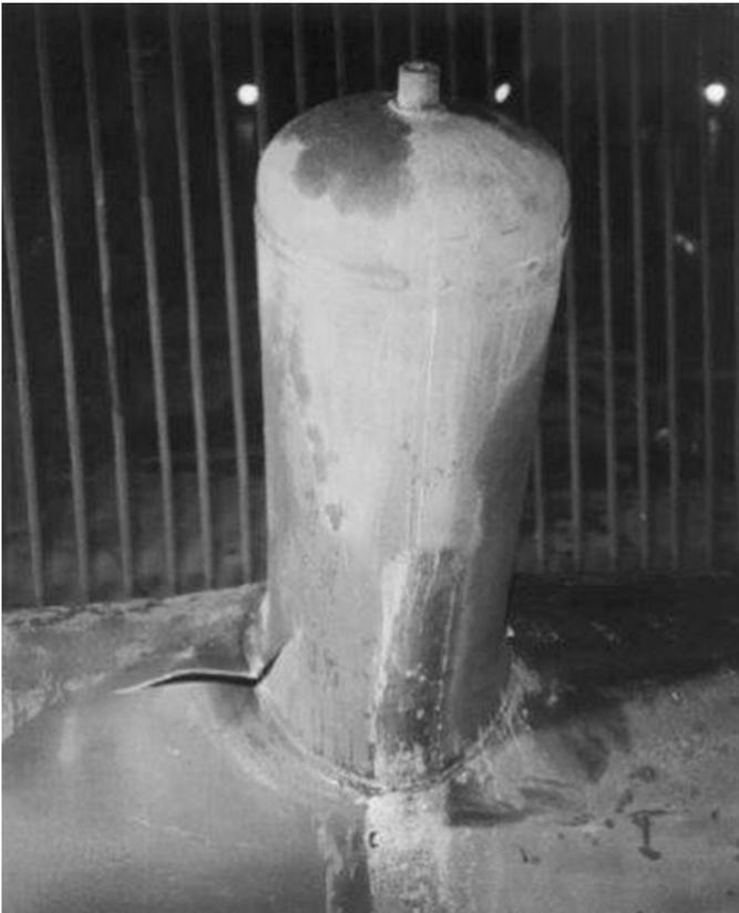
Fig. 7. Rupture of the test vessel
