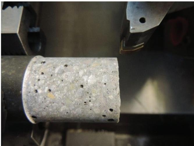
Fig. 3. The view of sample made of polymer concrete
