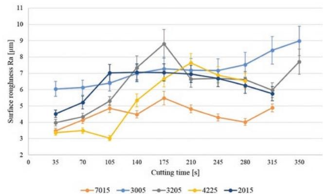
Fig. 7. The surface roughness Ra versus time
