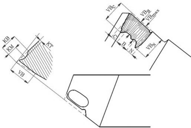
Fig. 1. Indicators of turning tool wear [8]
