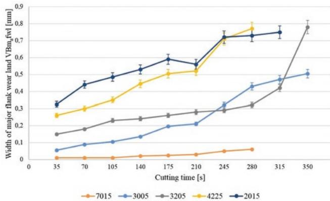
Fig. 4. The width of major flank wear land versus time
