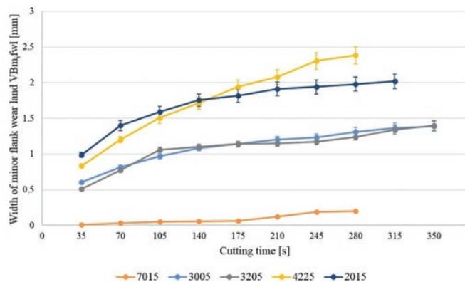
Fig. 5. The width of minor flank wear land versus time
