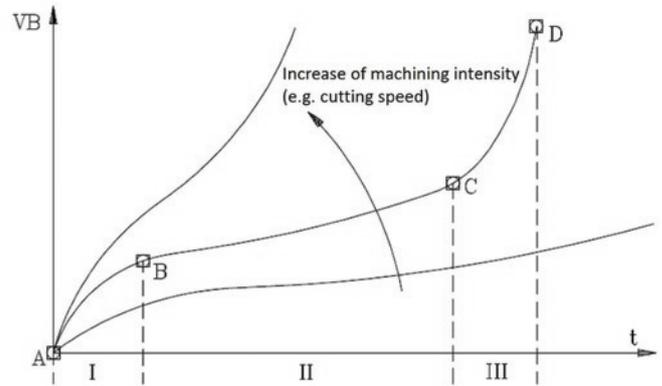
Fig. 2. Typical tool wear versus time [8]
