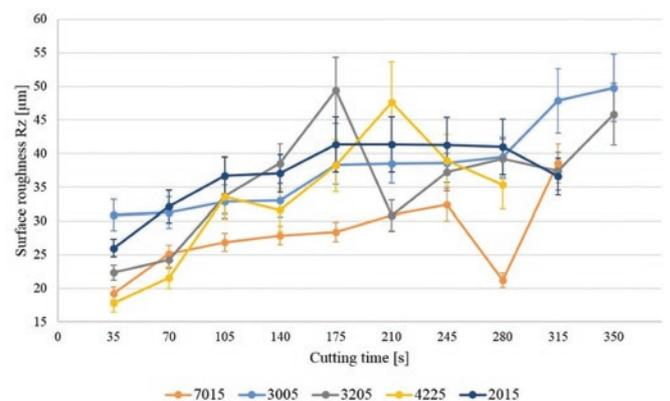
Fig. 8. The surface roughness Rz versus time
