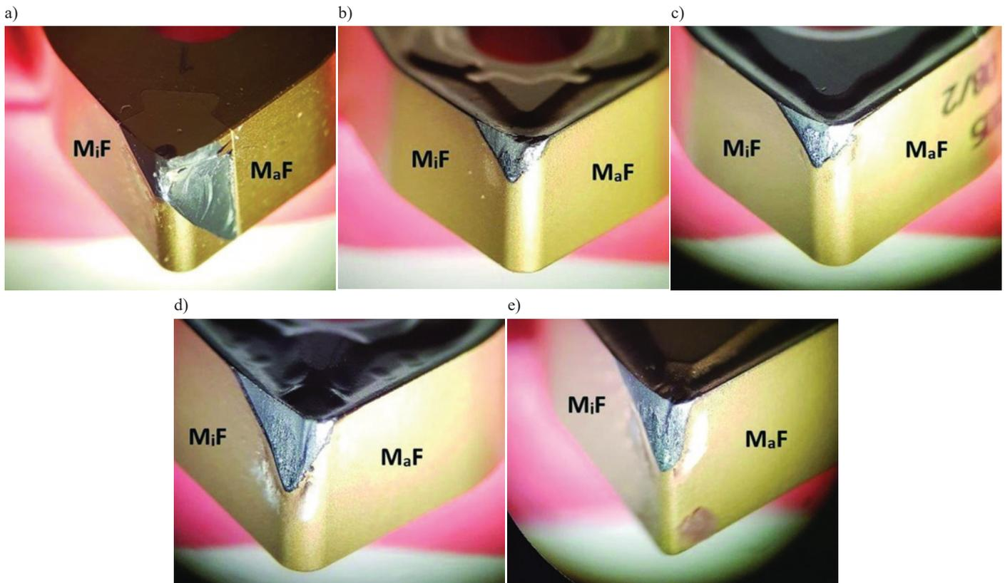
Fig. 9. Views of inserts after the machining a) WNGA 060408 S01030A 7015, b) WNMG 060408 KF 3005, c) WNMG 060408 KR 3205 d) WNMG 060408 PM 4225, e) WNMG 060404 WF 2015
