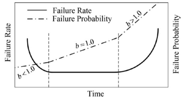
Fig. 1. Failure rates and Weibull parameter  $b$
