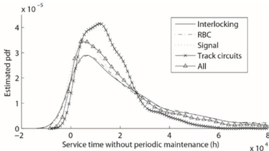
Fig. 8. Probability density function of the service time without periodic maintenance
