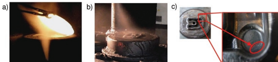
Fig. 3. Inappropriate lubrication: a) bad synchronization of the lubricating system with the forging process b) too intensive lubrication - no evaporation of the liquid from the lubricant mixture, c) crack in die inserts' corner – Rebinder effect
