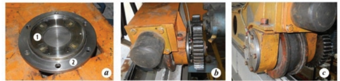
Fig. 6. Force transducer type HDT: a) components; b) HDT fitted in the driven wheel bearing housing - the cogwheel side; c) HDT fitted in the driven wheel bearing housing - the wall side
