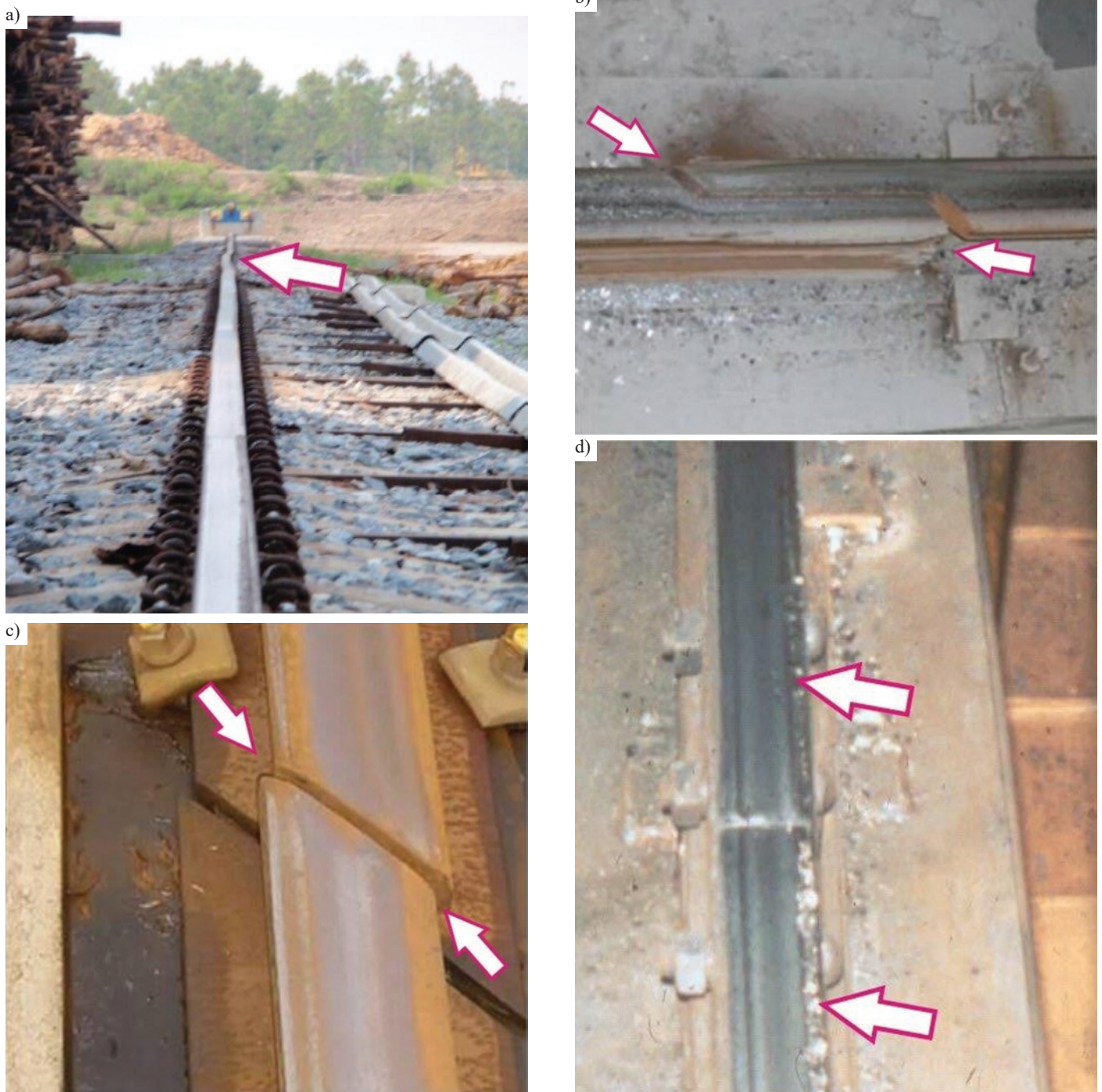
Fig. 3. (a-d) Examples of typical damage of crane runway rails
