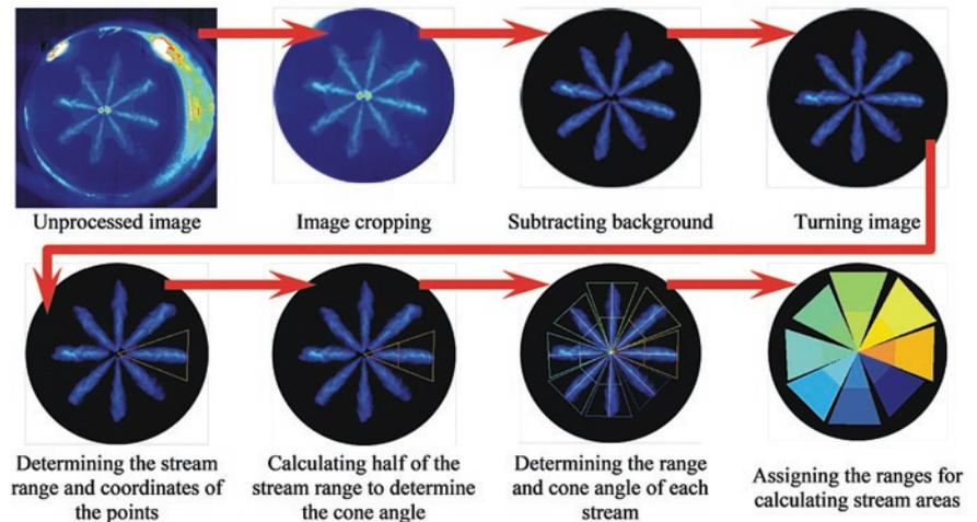
Fig. 3. Image processing and determining the geometric indicators of the fuel stream
