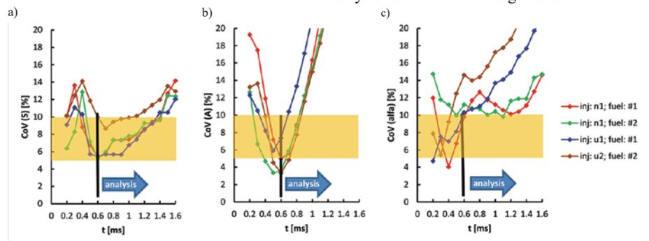
Fig. 7. Choice of analysis time for fuel spray coefficients based on the coefficient of variation: a) stream range – CoV (S), b) stream surface area – CoV (A), c) stream cone angle – CoV (alpha)
