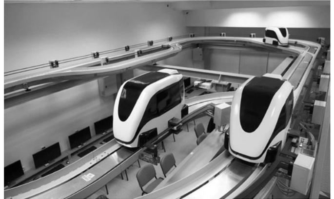
Fig. 3. Physical model of a PRT vehicle in a laboratory station
