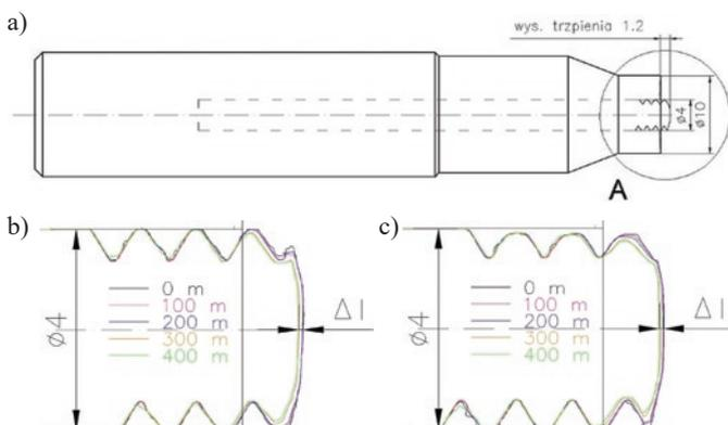
Fig. 7. The tool pin measurement results: a) characteristic dimensions b) 0°plane measurement c) 90° plane measurement
