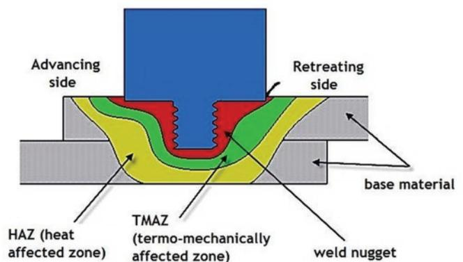
Fig. 2. The microstructure zones of the FSW process
