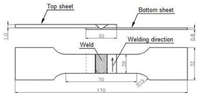
Fig. 4. Welded joint sample dimensions
