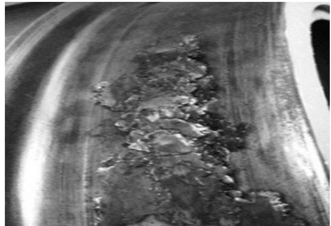
Fig. 2. Multi-layered metal scale of wheelset wheel
