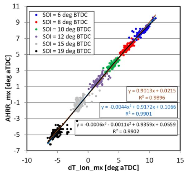
Fig. 14. The relation between the angle at maximum heat release rate ( $AHRR_{mx}$ ) and the angle at the maximum derivative of the thermal phase ( $dT_{Ion\_mx}$ ) for all test points
