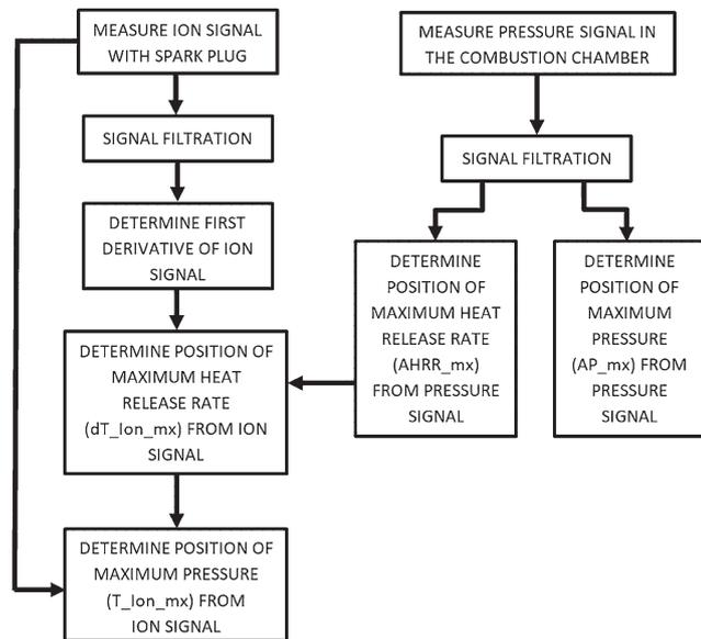
Fig. 9. Calculation algorithm that allows to determine the characteristic points of the ionization signal and its derivative
