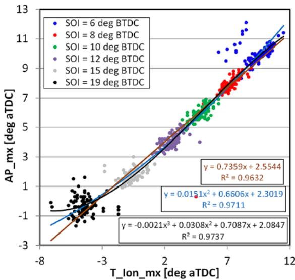
Fig. 11. The relation of the maximum pressure angle ( $AP_{mx}$ ) and the maximum value of the thermal ionization voltage angle ( $T_{Ion\_mx}$ ) including all test points
