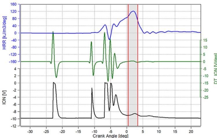
Fig. 10. The ionization signal analysis range (3° on the crankshaft) – marked in red
