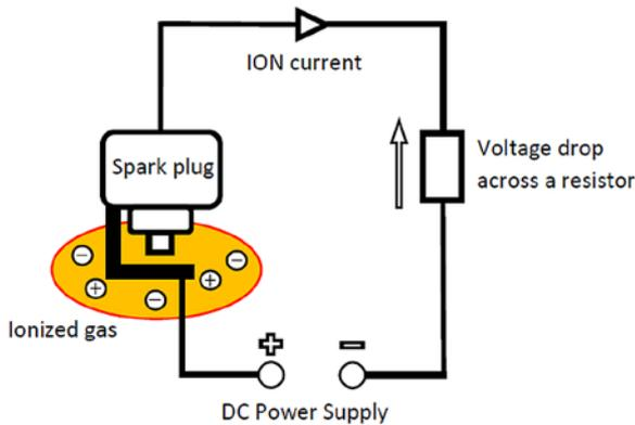
Fig. 1. Diagram of the ionization signal measuring circuit [7]
