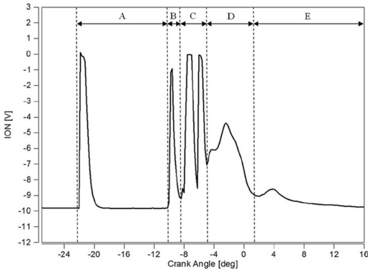
Fig. 8. The real ionization voltage signal along with markers indicating the different phases
