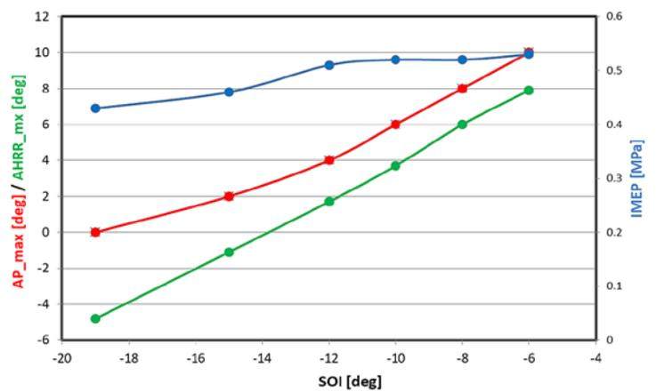
Fig. 6. Influence of start of ignition angle on the averaged values of: indicated mean effective pressure (IMEP), maximum cylinder pressure angle (AP\_max) and maximum heat release rate angle (AHRR\_mx) in a natural gas engine ( $\lambda = 1$ )
