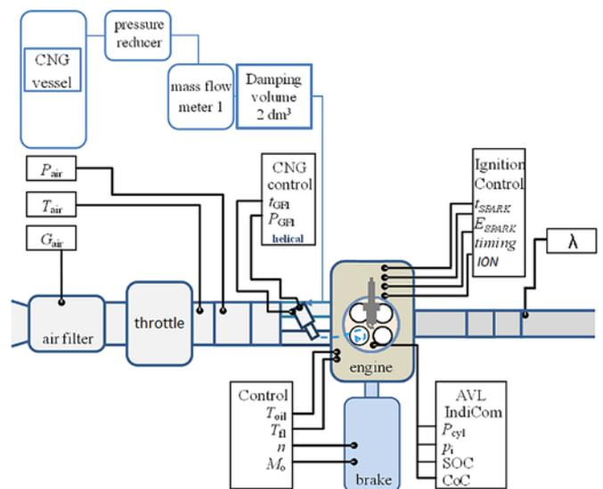
Fig. 4. Ionization signal measurement test bench schematic [7]
