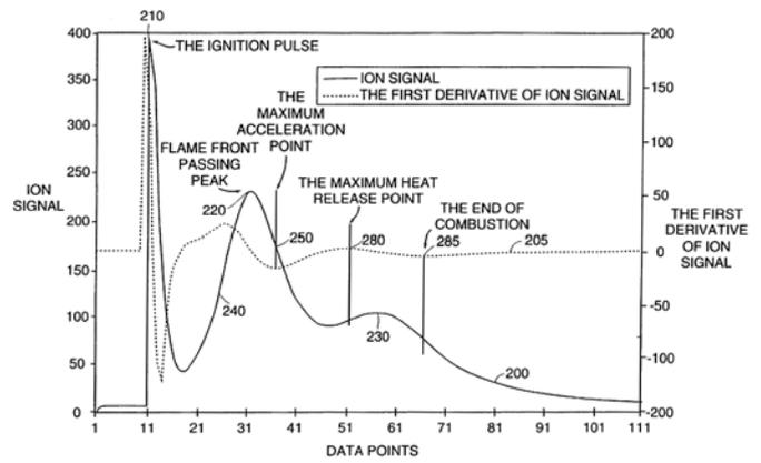
Fig. 2. The ionization voltage signal and its first derivative with the three phases marked [3]
