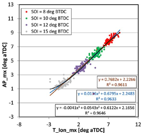
Fig. 13. The relation between the maximum pressure angle ( $AP_{mx}$ ) on the crankshaft angle at the maximum thermal ionization voltage ( $T_{Ion\_mx}$ ) after reducing the number of test points
