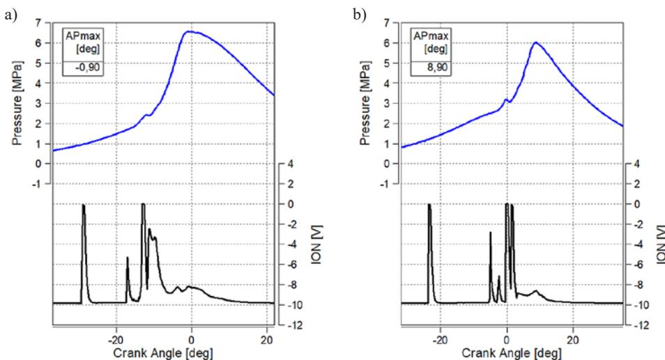
Fig. 7. The indicated pressure and ionization voltage signal characteristics from the combustion chamber for extreme measuring points still within the scope of the tests: a) SOI = 19 deg before TDC, b) SOI = 6 deg before TDC
