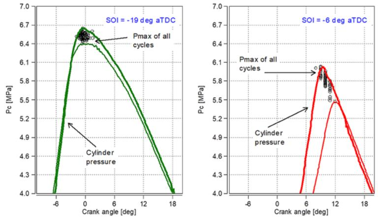
Fig. 12. Changes in the  $AP_{mx}$  angle value at the extreme ignition angle (SOI = 19 before TDC and 6 deg before TDC)
