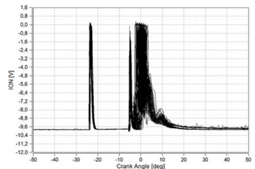
Fig. 3. The non-repeatability of in-cylinder processes: a) combustion pressure, b) ionization voltage signal for 100 consecutive engine cycles (mean indicated pressure IMEP = 0.5 MPa, ignition start crankshaft angle = 6 deg before TDC, excess air ratio  $\lambda = 1$ )
