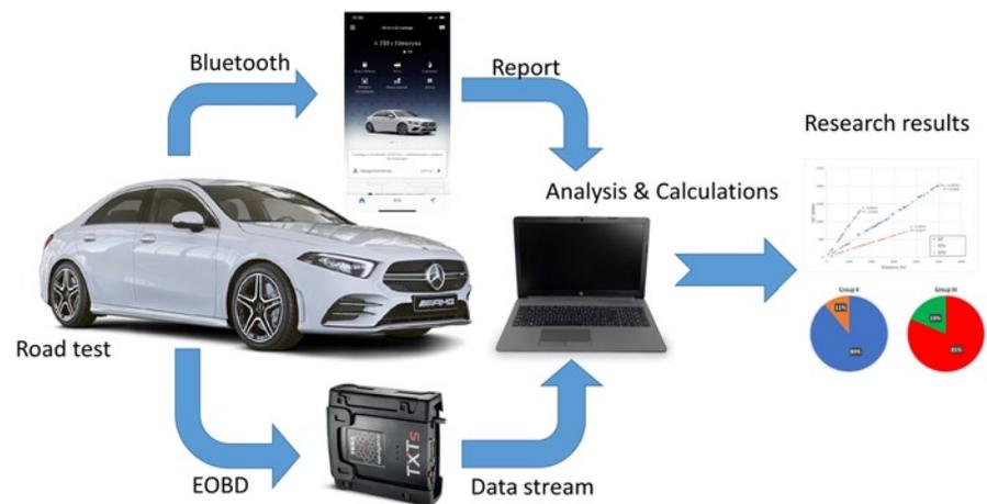
Fig. 1. Measurement system diagram
