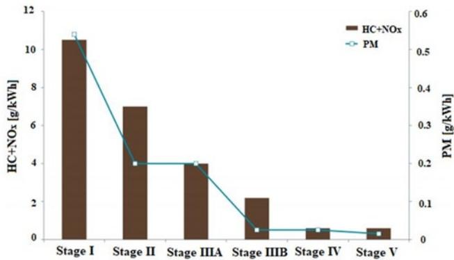
Fig. 1. Exhaust emission limit changes of HC+NO<sub>x</sub> and PM for the Stage I-V norms [11]
