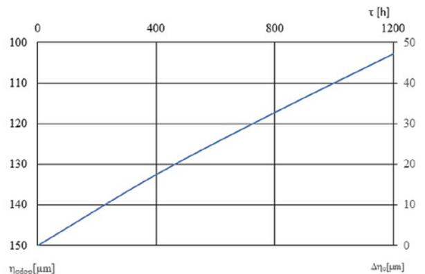
Fig. 7. Dependence of the permissible level  $\eta_{dop}$  and residual tolerance  $\Delta\eta = \eta_{gr} - \eta_{dop}$  on verification periodicity  $\tau$  for the total radial clearance in piston pairs [Source: Own study]
