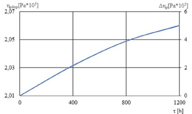
Fig. 6. Dependence of the permissible level  $\eta_{dop}$  and residual tolerance  $\Delta\eta = \eta_{gr} - \eta_{dop}$  on verification periodicity  $\tau$  for pump's maximum pressure [Source: Own study]
