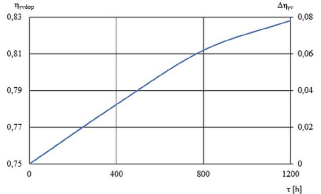
Fig. 5. Dependence of the permissible level  $\eta_{dop}$  and residual tolerance  $\Delta\eta = \eta_{gr} - \eta_{dop}$  on verification periodicity  $\tau$  the pump's volumetric efficiency factor [Source: Own study]
