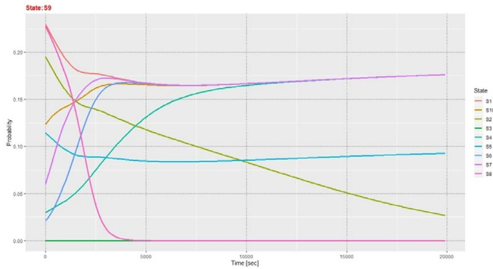
Fig. 6. Relationship between the transition probability from Refuelling state and its duration
