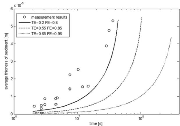
Fig. 12. Results of measurements and simulations for different transfer efficiency  $TE$  and filter efficiency  $F_E$
