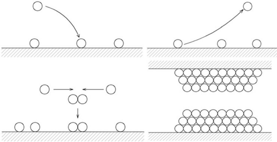
Fig. 3. Elementary stages of deposition model a) deposition, b) resuspension, c) agglomeration, d) clogging
