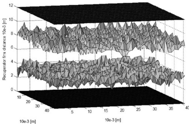
Fig. 10. Sediments on recuperator fins after 12e7 iterations
