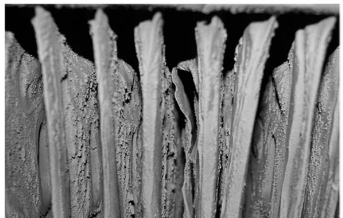
Fig. 2 Recuperator fins contaminated with overspray sediments
