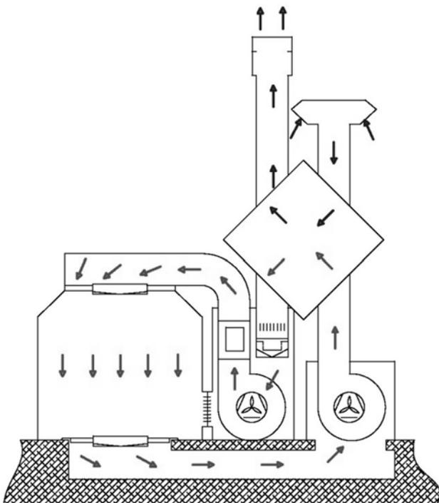
Fig. 1 A location of the heat exchanger in typical booth assembly
