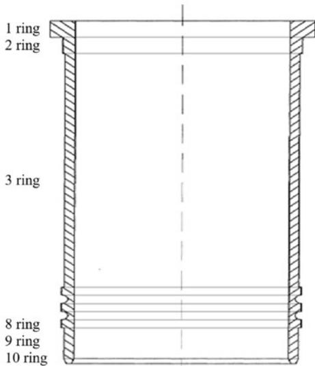
Fig. 1. Cylinder liner decomposition for the 4Cz 8,5/11 type engine
