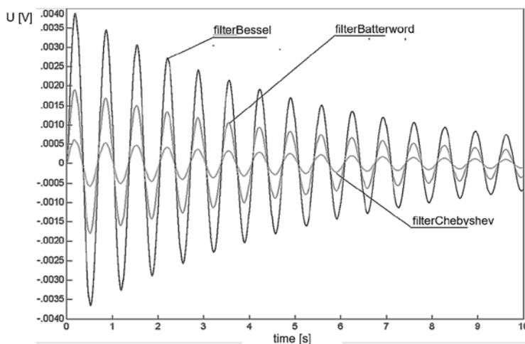
Fig. 5. Results of vibration damping effectiveness of a cylinder liner of the 4Cz8,5/11 type engine obtained using different filters
