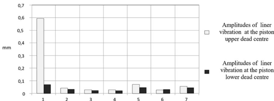
Fig. 8. Amplitudes of cylinder liner vibrations measured during the experiment
