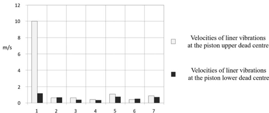
Fig. 9. Velocities of cylinder liner vibrations measured during the experiment
