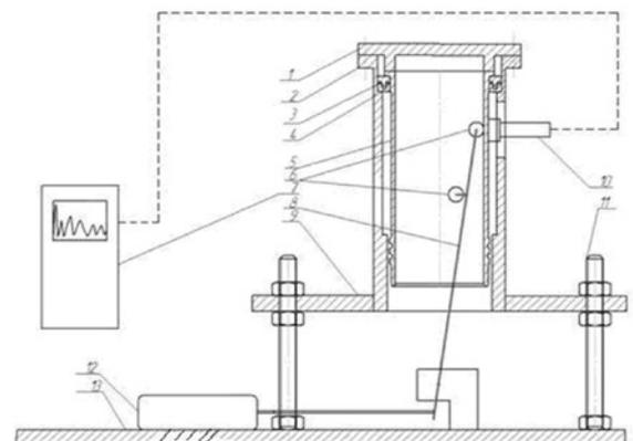
Fig. 7. Experimental stand for simulation studies of cylinder liner of the 4Cz 8,5/11 type engine vibration parameters 1 – cylinder head; 2 – cylinder coat; 3 – upper clamping ring; 4 – lower clamping ring; 5 – liner; 6 – upper and lower firing pin; 7 – vibrometer TV-300; 8 – bolt; 9 – support plate; 10 – TSV-01 vibration detector; 11 – screws; 12 – vibrator; 13 – base plate
