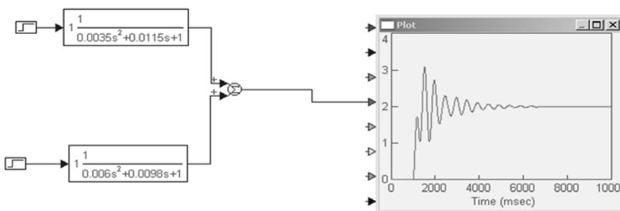
Fig. 4. A diagram of a functional model of a cylinder liner of the 4Cz8,5/11 type engine in the Vis Sim environment
