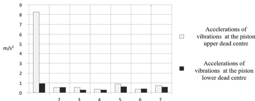
Fig. 10. Accelerations of cylinder liner vibrations measured during the experiment
