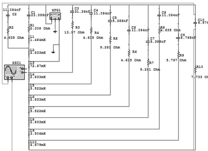
Fig. 3. A diagram representing a cylinder liner of a 4Cz 8,5/11 type engine in the form of an electric network
