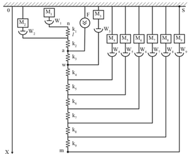
Fig. 2. A diagram of a mechanical representation of a cylinder liner of a 4Cz8,5/11 type engine in the form of a two-terminal network
