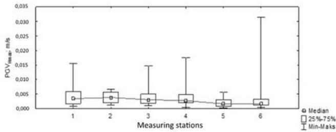
Fig. 6. Distribution of the medians of the horizontal component value of peak ground vibrations velocity for measurement stations for tremors with energy  $E \geq 106 J$  occurred in 2010 - 2014.
