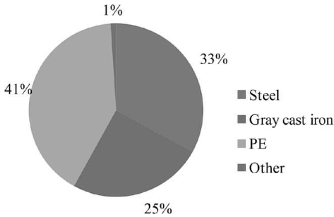
Fig. 2. The material composition of water supply system in 2014. On the graphs: "Other" – asbestos and PVC
