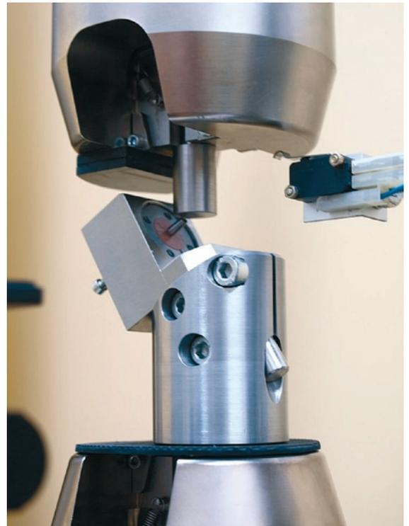
Fig. 6. Test stand according to PN-EN ISO 14801 standard – clamping set with the resin cylinders with embedded implants mounted in holder of fatigue testing machine (Instron 8874)
