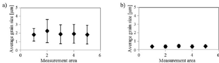
Fig. 10. The average diameter of the  $\gamma'$  reinforcing phase into the leading edge: a) blade No. 2, b) blade No. 4
