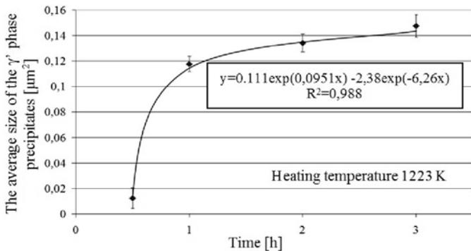
Fig. 4. Changes in the average size of the  $\gamma'$  phase particles depending on the heating time of samples of the blades at the temperature of 1223K
