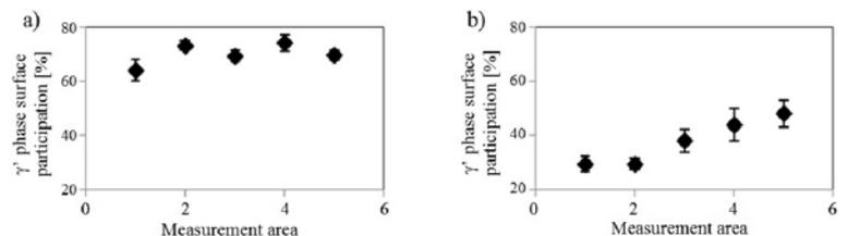
Fig. 9. Surface participation of the  $\gamma'$  reinforcing phase into the leading edge: a) blade No. 2, b) blade No. 4
