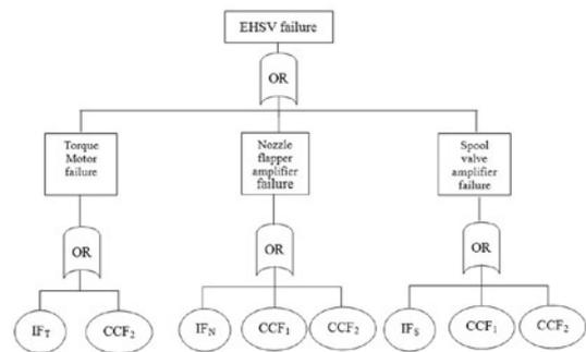
Fig. 5. The fault tree of EHSV with CCF
