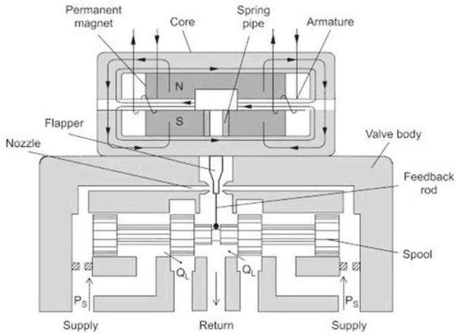
Fig. 1. The schema of EHSV
