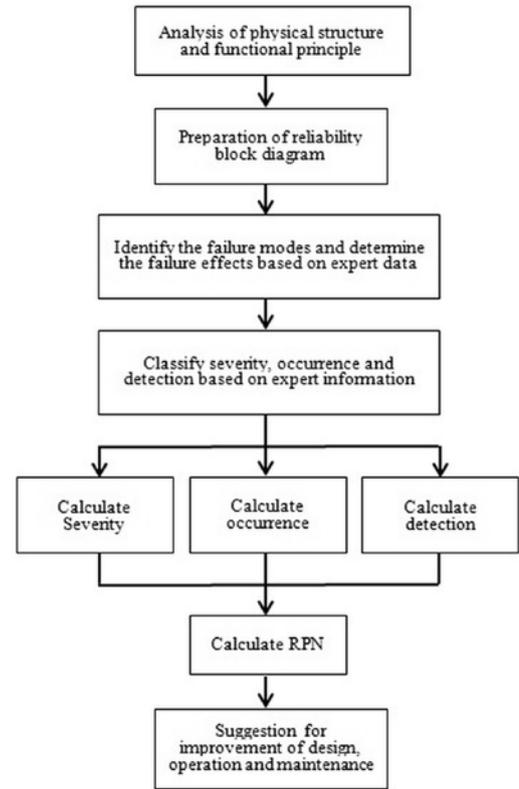
Fig. 3. The framework for FMECA of EHSV
