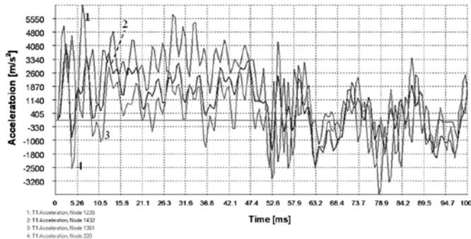
Fig. 18. Longitudinal accelerations in selected points of the tank body after a hit of a non-piercing missile: 1 – tower centre of mass, 2 – tank body centre of mass, 3 – a driver, 4 – floor under a driver's seat
