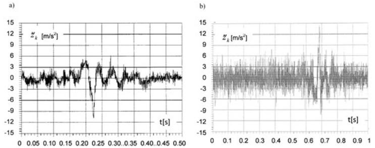
Fig. 7. Courses of vertical body accelerations, crossing a triangle prism of a height of 170mm and length of  $l_0$  at the speed  $v=5.56\text{m/s}$ : a) and b) reflect various conditions of a caterpillar chassis
