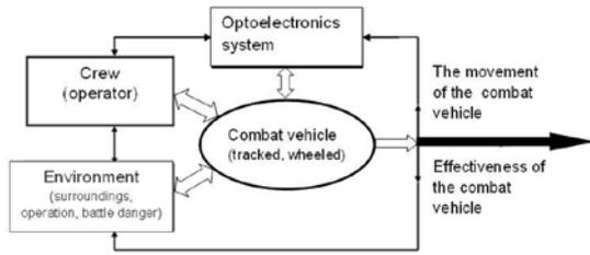
Fig. 1. Diagram of interactions in the system: combat vehicle – human – internal equipment – surroundings a) dynamic overcoming of a slope [3], b) overcoming of a cross ditch
