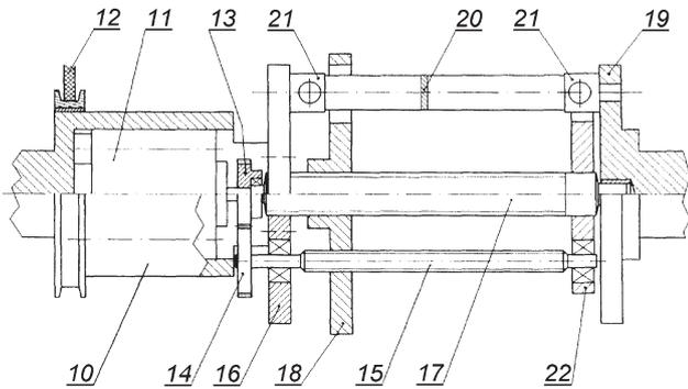
Fig. 2. Flexible coupling
