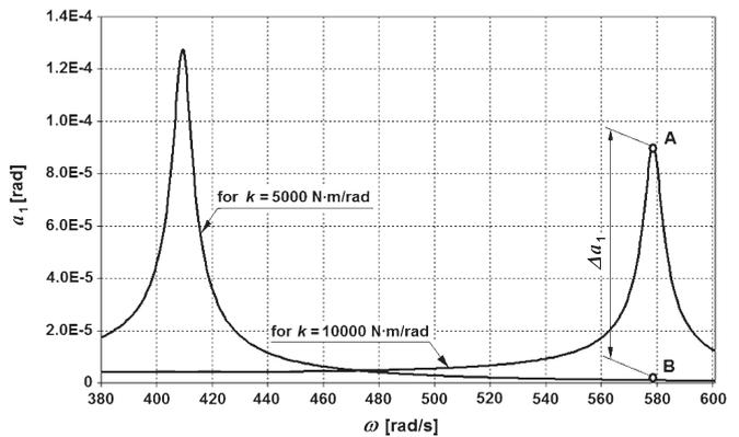
Fig. 4. The graph of amplitude  $a_1$  in relation to extortion  $\omega$  frequency for torsional stiffness  $k = 10000 \text{ N} \cdot \text{m}/\text{rad}$  and  $k = 5000 \text{ N} \cdot \text{m}/\text{rad}$
