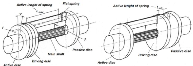
Fig. 1. The scheme of actions of flexible coupling
