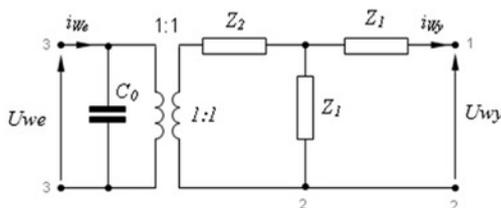
Fig. 9. The transformed substitute circuit of the input piezoelectric plate
