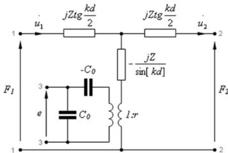
Fig. 5. The equivalent Mason circuit of piezoelectric plate
