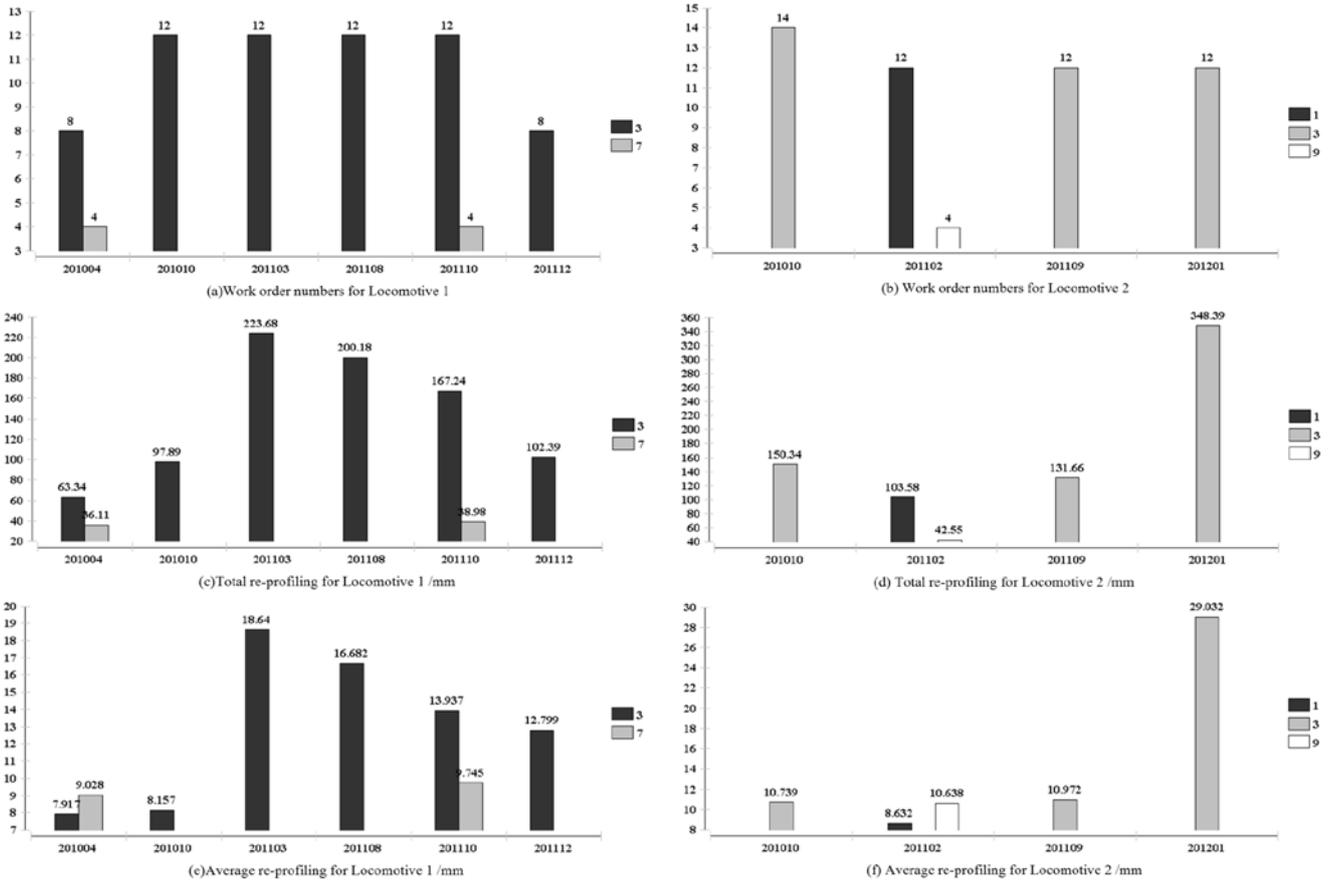
Fig. 5. Work order statistics on re-profiling by date
