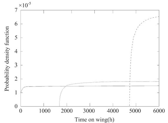
Fig. 3. The changing trend of the probability density function of sudden failures (The solid line shows the first phase, the dotted line shows the second phase and the dashed line shows last phase)
