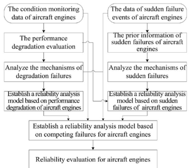
Fig 1. The flow diagram of reliability evaluation for aircraft engines based on competing failures
