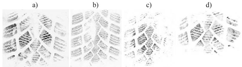
Fig. 12. Uniroyal Rallye 680 tread prints: - tire pressure 2.2 bar - load: a - 1841 N, b - 3682 N; - load 614 N - tire pressure: c - 1.5 bar, d - 3 bar
