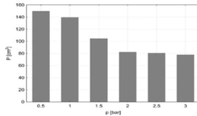
Fig. 13. Changing the area of contact as a function of the pressure in the tire at a constant load.
