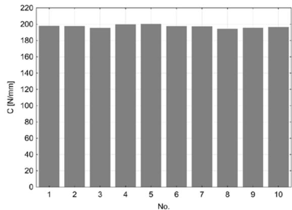
Fig. 4. Bar graph showing the designated values of radial tire stiffness from 10 repetitions
