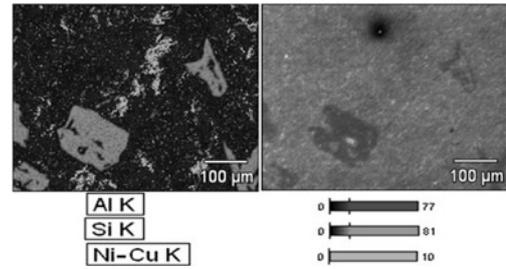
Fig. 2. Depiction of AISi21CuNi surface from SEM microscope and a map of chemical elements distribution for this alloy
