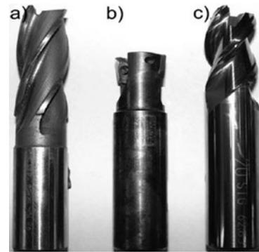
Fig. 3. Tools that were used for machining: a) NFPa, b) R390-020B20-11L, c) E5423200
