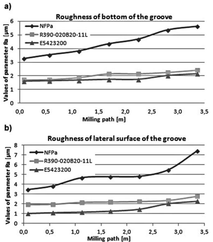
Fig. 6. Surface roughness of: a) bottom of the groove, b) lateral surface of the groove (machining parameters for mills: NFPa – P1; R390-020B20-11L – P2; E5423200 – P3 according to Table 2)
