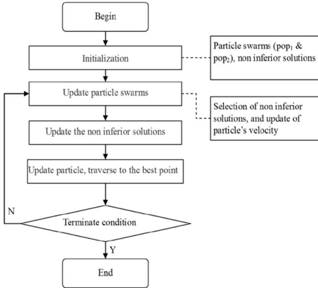
Fig. 3. Procedure of rules based MOPSO solution algorithm
