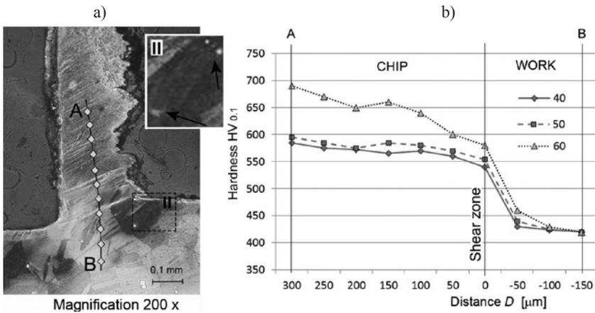
Fig. 5. Chip creation zone with titanium carbide particles indicated by arrows (a) and micro-hardness distribution along AB line for the feed  $f = 0.1$  mm and cutting speed  $v_c = 40; 50; 60$  m/min (b)
