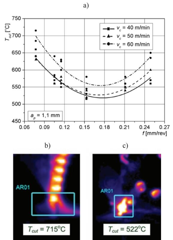
Fig. 4. Temperature of tool wedge: a)  $T_{cut} = f(f, v_c)$ , b) infra-red photo for  $v_c=60 \text{ m/min}$  and  $f=0.08 \text{ mm/rev}$ , c) infra-red photo for  $v_c=40 \text{ m/min}$  and  $f=0.15 \text{ mm/rev}$
