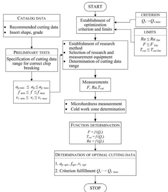
Fig. 1. Scheme of the productivity improvement procedure during turning ( $Q_v \max$ )
