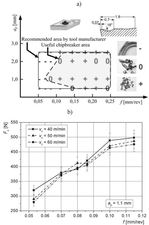
Fig. 3. Classification of chips forms with useful chipbreaker area type SM in local testing environment for  $v_c=50 \text{ m/min}$ , (a) and influence of feed on cutting force (b)
