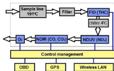
Fig. 3. Schematics of the Semtech DS analyzer
