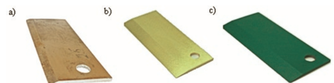
Fig. 3. Test knives: a) steel NC6, b) TiN coated, c) AS48 coated
