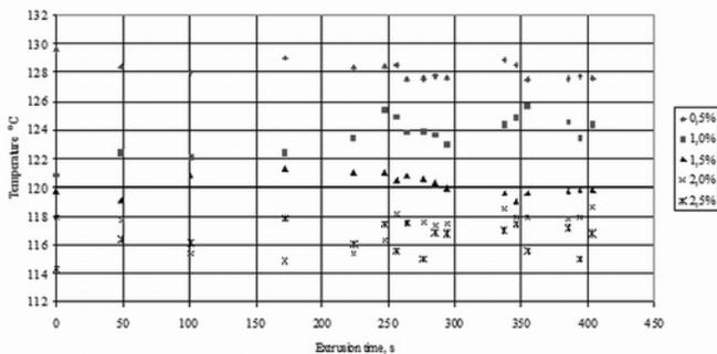
Fig. 10. Dependence temperature of nozzle head on extrusion time with screw rotational speed  $v^5 = 1.85 \text{ s}^{-1}$  and content of microspheres range  $0 \div 2.5\% \text{ mass}$ .
