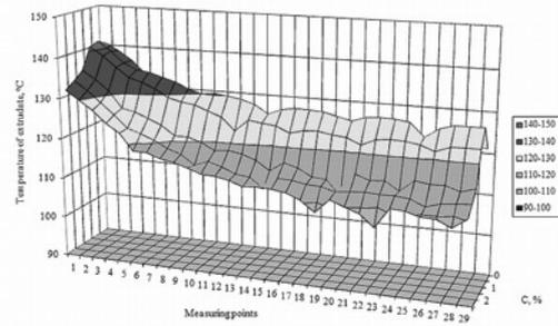
Fig. 5. Dependence of the extrudate temperature in individual measuring points at a rate of screw rotation  $v^4 = 1.57 \text{ s}^{-1}$  and the content of microspheres from 0 to 2.5% of the masses.
