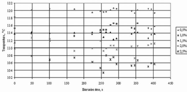
Fig. 8. Dependence temperature of nozzle head on extrusion time with screw rotational speed  $v^3 = 1.30 \text{ s}^{-1}$  and content of microspheres range  $0 \div 2.5\% \text{ mass}$ .
