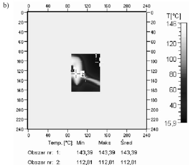
Fig. 1. Examples of thermal images extrusion head and micro brewing: a) with the selected section of the extrudate surface measurement, b) with the selected measurement points on the surface of the nozzle head, and extrudate.
