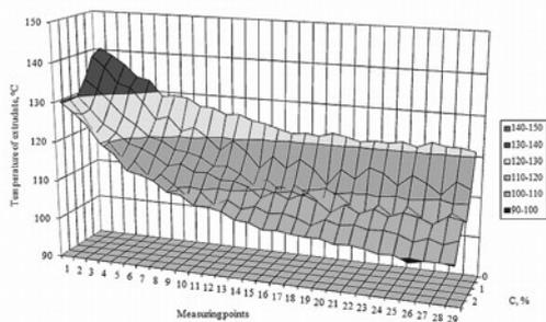
Fig. 2. Dependence of the extrudate temperature in individual measuring points at a rate of screw rotation  $v^1 = 0.75 \text{ s}^{-1}$  and the content of microspheres from 0 to 2.5% of the masses.
