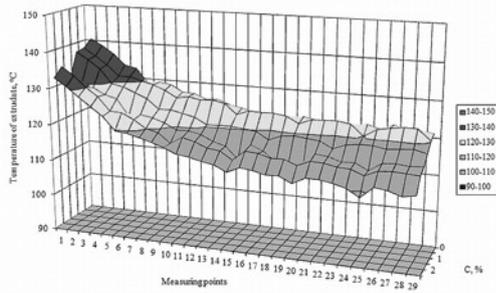
Fig. 4. Dependence of the extrudate temperature in individual measuring points at a rate of screw rotation  $v^3 = 1.30 \text{ s}^{-1}$  and the content of microspheres from 0 to 2.5% of the masses.
