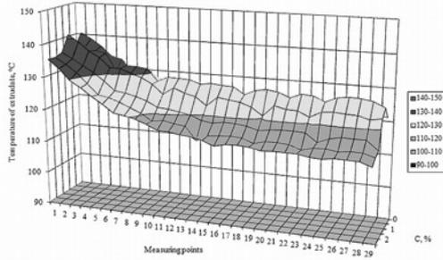
Fig. 6. Dependence of the extrudate temperature in individual measuring points at a rate of screw rotation  $v^3 = 1.85 \text{ s}^{-1}$  and the content of microspheres from 0 to 2.5% of the masses.
