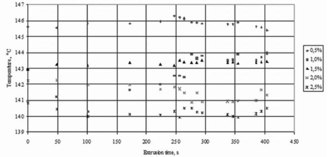
Fig. 7. Dependence temperature of nozzle head on extrusion time with screw rotational speed  $v^1 = 0.75 \text{ s}^{-1}$  and content of microspheres range  $0 \div 2.5\% \text{ mass}$ .
