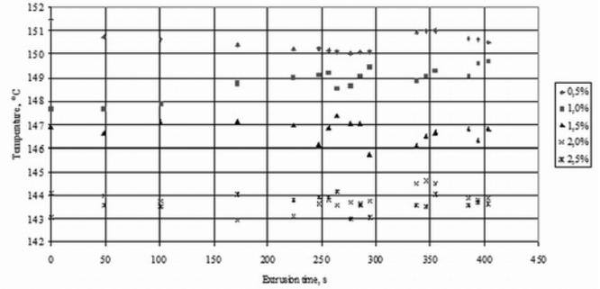
Fig. 9. Dependence temperature of nozzle head on extrusion time with screw rotational speed  $v^4 = 1.57 \text{ s}^{-1}$  and content of microspheres range  $0 \div 2.5\% \text{ mass}$ .
