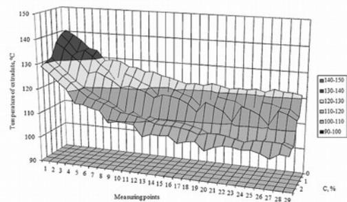
Fig. 3. Dependence of the extrudate temperature in individual measuring points at a rate of screw rotation  $v^2 = 1.02 \text{ s}^{-1}$  and the content of microspheres from 0 to 2.5% of the masses.
