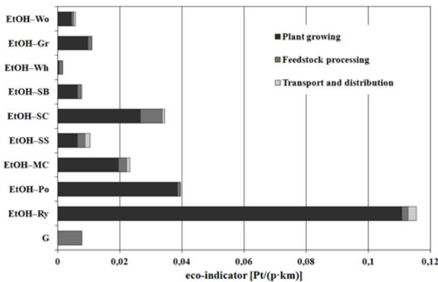
Fig. 5. Environmental impact assessment of the fuel preparation processes as obtained from the Eco-indicator 99 method
