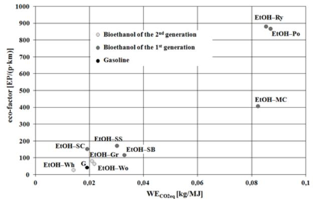
Fig. 6. Comparison between the energy-related GHG emission indicator and eco-factor values determined for the processes of preparation of the fuels under consideration
