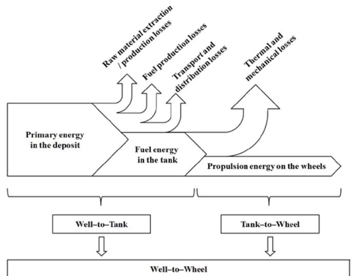
Fig. 1. Schematic diagram of individual stages of the Well-to-Wheel analysis
