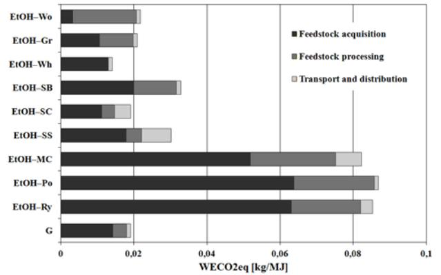
Fig. 3. Energy-related GHG emission indicator determined for the stage of preparation of the fuels under consideration
