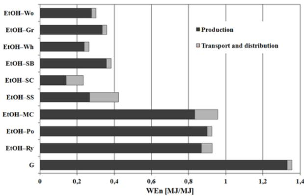
Fig. 2. Total amount of non-renewable energy used to prepare fuel of 1 MJ energy content
