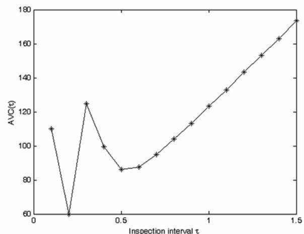
Fig.5. Average long-run maintenance cost rate versus inspection interval  $\tau$  with  $C_i=20$
