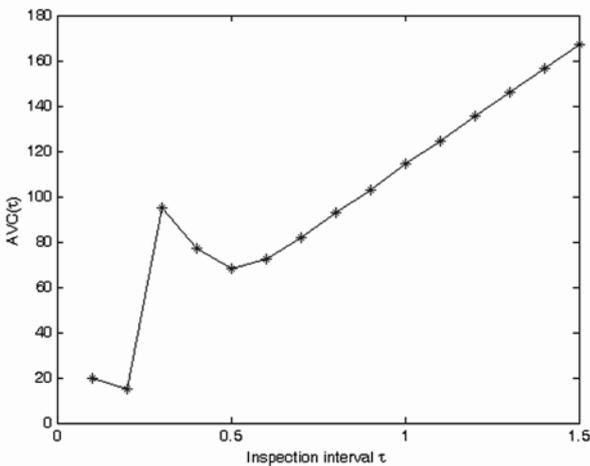
Fig.3. Average long-run maintenance cost rate versus inspection interval  $\tau$  with  $C_i=1$
