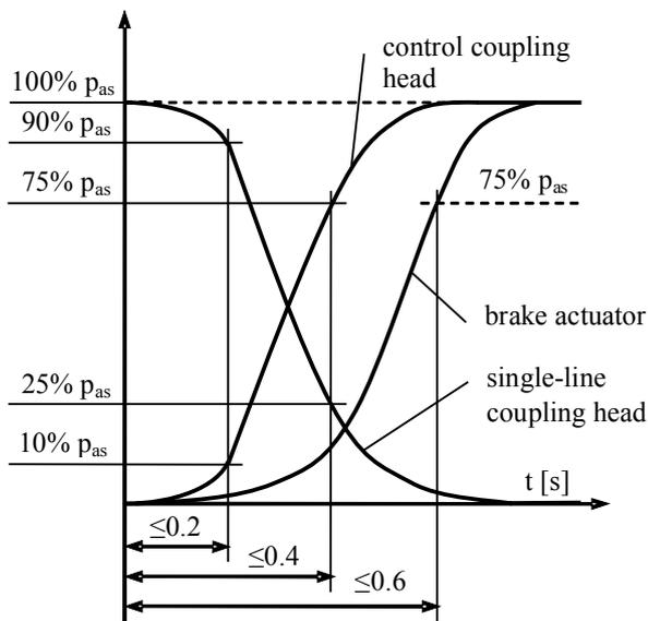
Fig.2. Variation in pressure as a function of time and the required response times of the tractor control unit
