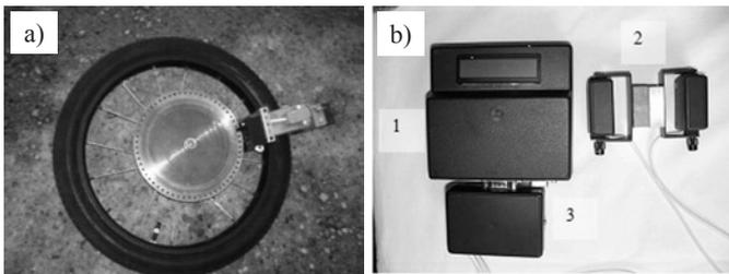
Fig. 4. Devices for measuring the braking distance and braking deceleration: a – fifth wheel pulse disc with an optical sensor; b – decelerometer components: 1 – microcontroller; 2 – measuring sensors; 3 – signal amplifier
