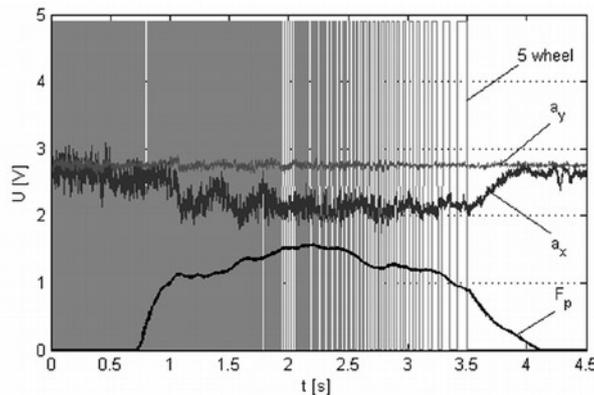
Fig. 12. An example of using the measuring system in braking efficiency tests
