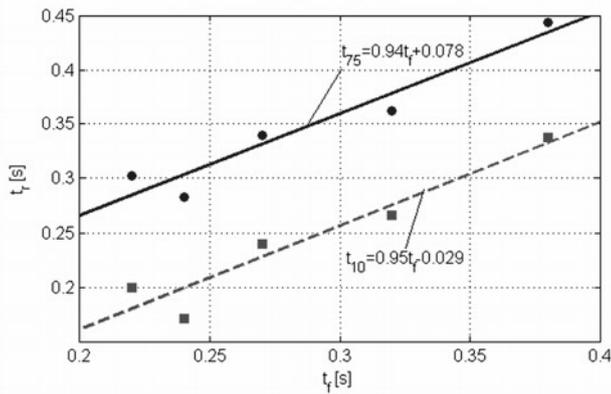
Fig. 11. The effect of the brake pedal force increase time  $t_f$  on the response time  $t_{75}$  ( $R^2=0.9275$ ) and  $t_{10}$  ( $R^2=0.9122$ ) of the dual-line braking system
