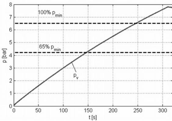
Fig. 8. Example variation of the increase in pressure  $p_v$  in the  $V=60.38 \text{ dm}^3$  substitute reservoir during the compressor capacity test.
