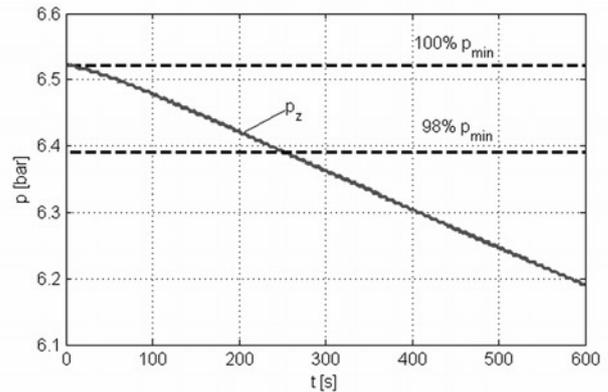
Fig. 5. Testing the air system leakage based on the variation of pressure  $p_z$  at the supply coupling head
