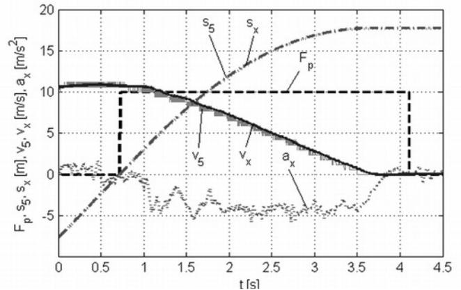
Fig. 13. Example measurement result obtained in the service braking system efficiency test:  $F_p$  – brake pedal force indicator;  $s_5, v_5$  – distance and velocity as determined from the fifth wheel measurements;  $a_x, v_x, s_x$  – acceleration, velocity and distance, as determined from the electronic decelerator measurements
