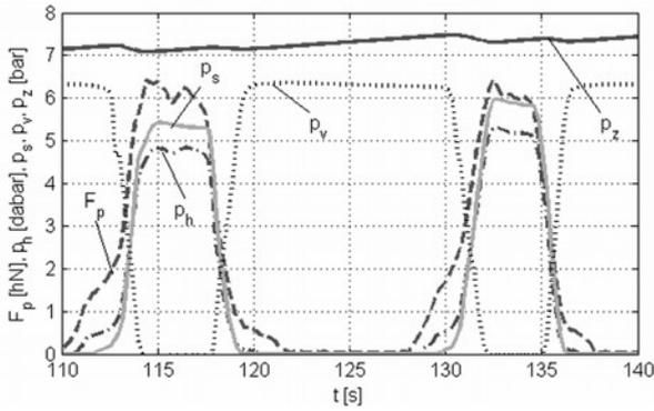
Fig. 7. Example variations of measured quantities during testing the air system coupling head pressure:  $F_p$  – brake pedal force;  $p_s, p_z, p_v$  – control, supply and single-line coupling head pressure, respectively;  $p_h$  – service brake system hydraulic pressure
