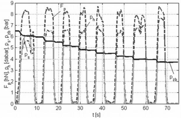
Fig. 9. Example variation of quantities recorded during testing the capacity of the compressed air reservoir in the dual-line system;  $F_p$  – brake pedal force,  $p_h$  – hydraulic system pressure,  $p_s$  – control coupling head pressure,  $p_{zb}$  – reservoir pressure
