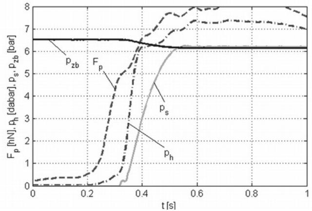
Fig. 10. Example variation of the quantities recorded during testing the tractor response time in the dual-line system:  $F_p$  – brake pedal force,  $p_h$  – hydraulic system pressure,  $p_s$  – control coupling head pressure,  $p_{zb}$  – reservoir pressure
