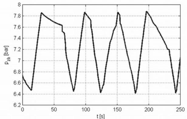
Fig. 6. Example variation of pneumatic system reservoir pressure  $p_{zb}$  during testing of the Visteon 51 10 018 unloader valve
