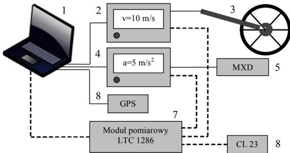
Fig. 3. Schematic of the measuring system for testing the vehicle braking process: 1 – portable computer; 2 – "fifth wheel" controller; 3 – fifth wheel; 4 – electronic decelerometer; 5 – MXD7202 acceleration sensor; 6 – Holux GPSlim 236 GPS receiver; 7 – LTC1286 measuring module; 8 – CL23 brake pedal pressure sensor
