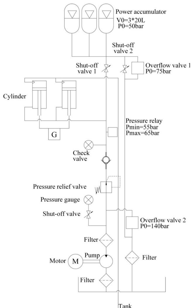
Fig. 4 Spindle carrier balance circuit of CNC machining center
