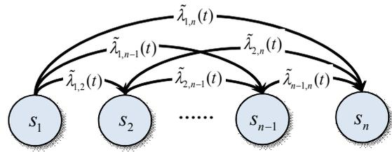
Fig. 3 The fuzzy state transition diagram for a non-repairable system
