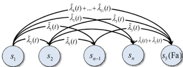
Fig. 6 State transition diagram of the spindle circuit of hydraulic system
