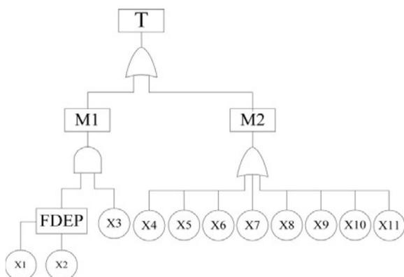
Fig. 5 Dynamic fault tree of the hydraulic system
