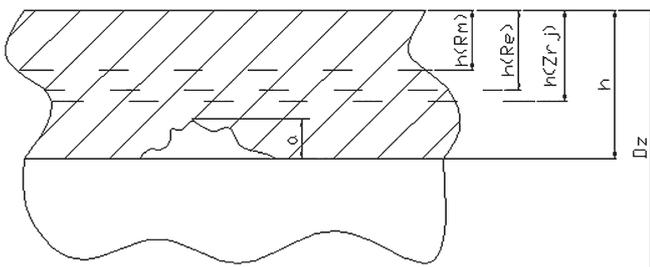
Fig. 1. Pipeline wall with example of corrosion pit and required limiting thicknesses
