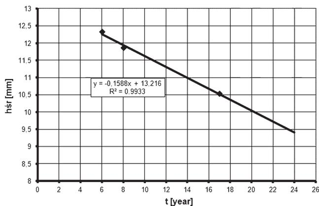
Fig. 5. Change in time of the pipe wall thickness  $h_{sr}$  for tested pipeline
