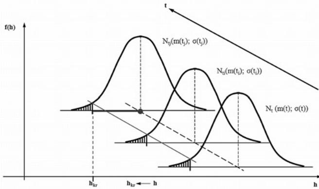
Fig. 3. Calculation of the time of limiting state on assumed probability level
