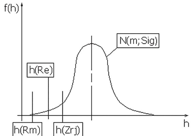
Fig. 2. Density function of the wall thicknesses distribution with required limiting thicknesses
