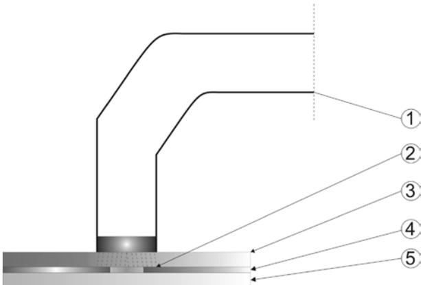
Fig. 2. Production of samples made of light-cured composites: 1 – lamp, 2 – exposed composite sample, 3 and 5 – plexiglass plates, 4 – steel form
