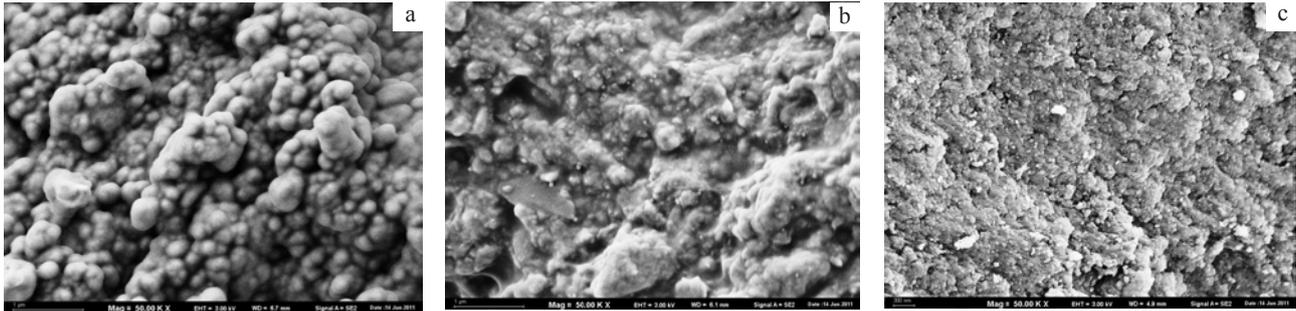
Fig. 1. SEM images of the sections of the studied materials: a) Filtek Silorane, b) Ice, c) Venus
