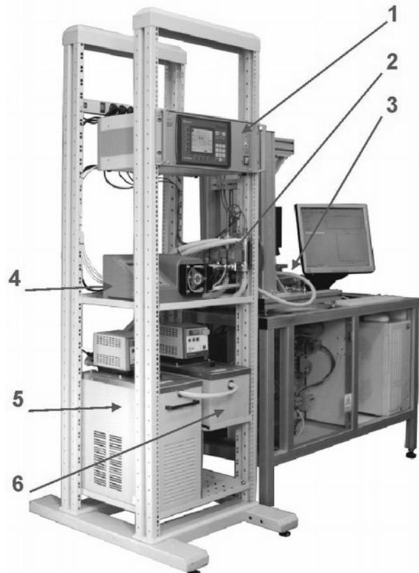
Fig. 3. Experimental stand for durability studies with specific thermal shocks module components: 1 – micro-processor control system, 2 – control valves, 3 – chewing simulator, 4 – peristaltic pump, 5 – cooling thermostat, 6 – heating ultra-thermostat
