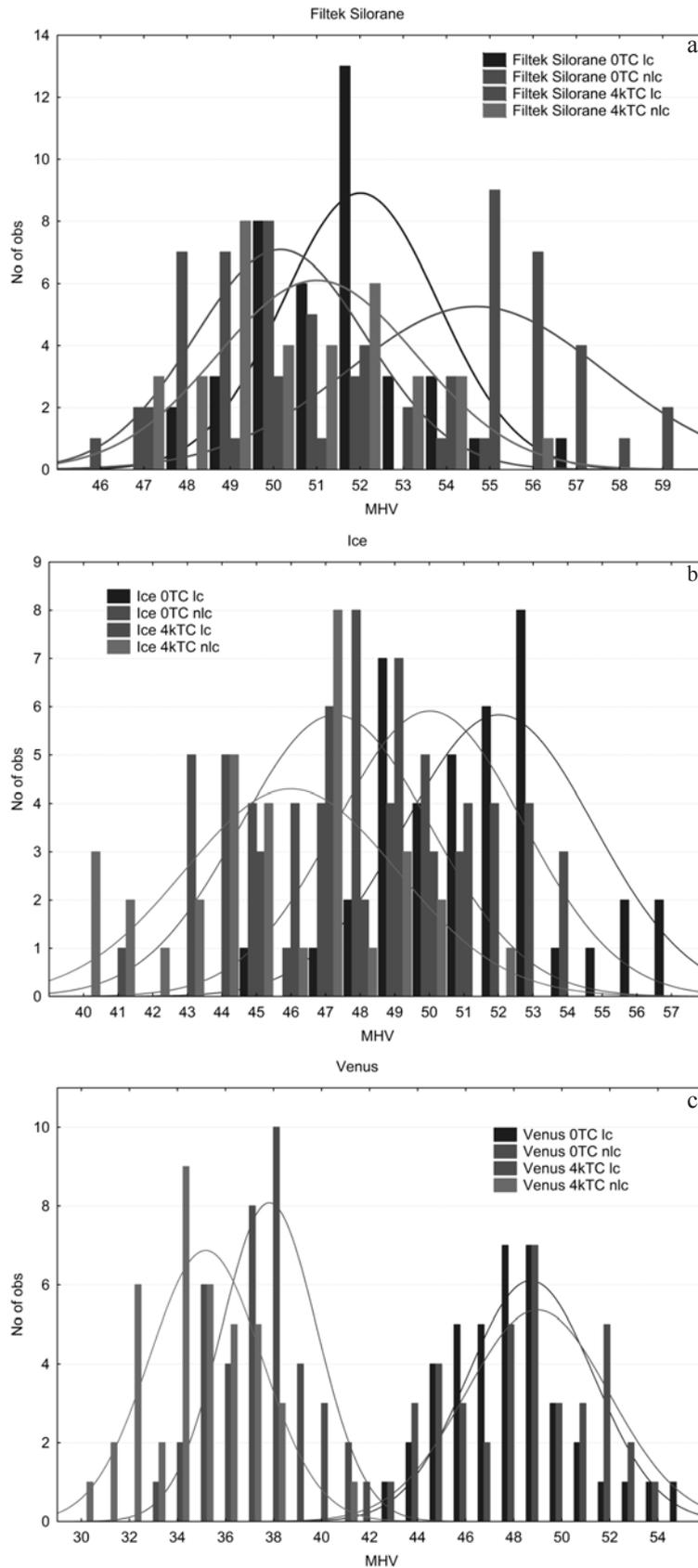
Fig. 5. Stemplot of micro-hardness of the studied materials after fatigue tests: a) Filtek Siloran, b) Ice, c) Venus
