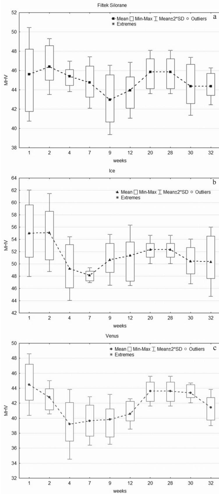
Fig. 6. Relationship of micro-hardness of the studied materials and ageing time in saline: a) Filtek Silorane, b) Ice, c) Venus
