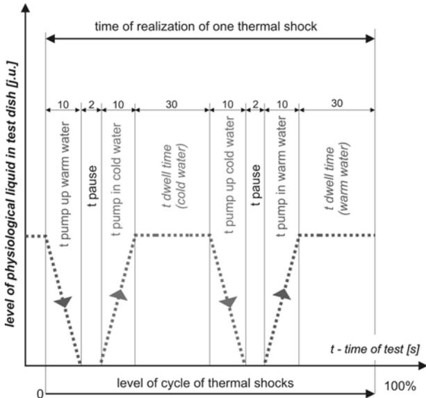
Fig. 4. Thermal shock algorithm with a single pumping of the operating liquid
