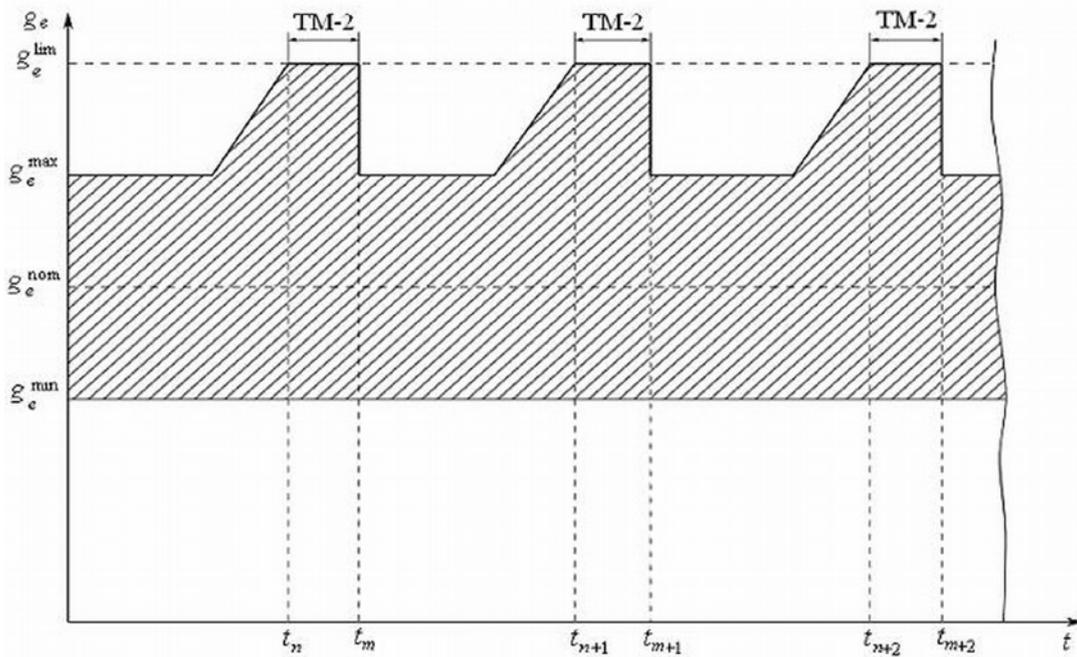
Fig. 2. Technical maintenance performance times according to comparative fuel consumption on the diesel locomotives
