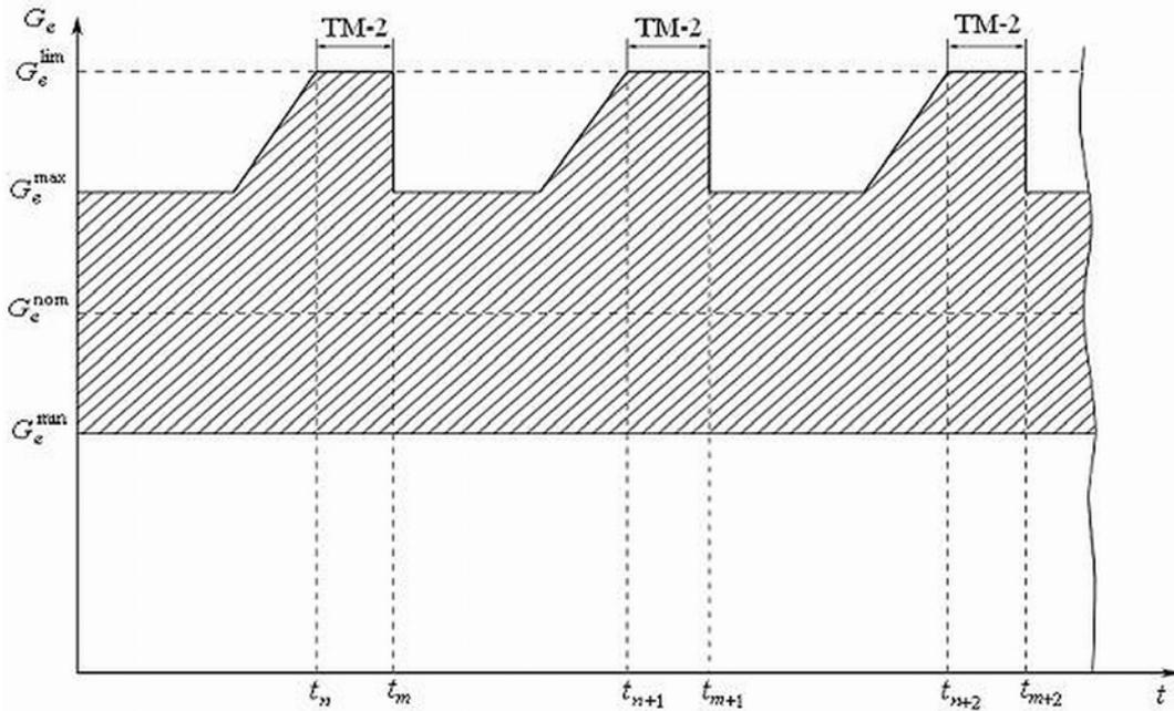
Fig. 1. Technical maintenance performance times according to fuel consumption per hour of the thermo diesels
