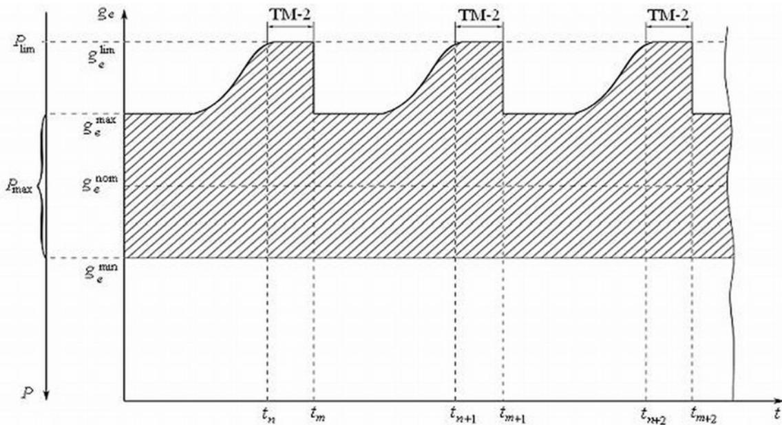
Fig. 4. Dependency of technical maintenance performance dates of diesel locomotives on comparative consumption of fuel and operating without failures probability
