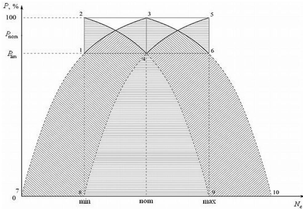
Fig. 3. Dependency of probability working without failures on the effective capacitance of diesel locomotives
