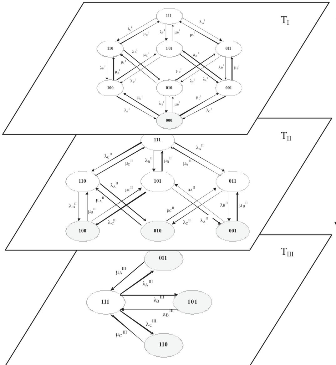
Fig. 6. A diagram of a reliability model with fixed phase duration [11]
