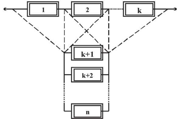
Fig. 1. A block diagram of a threshold structure
