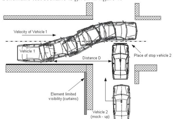
Fig. 1. Schematic scenario of an accident situation
