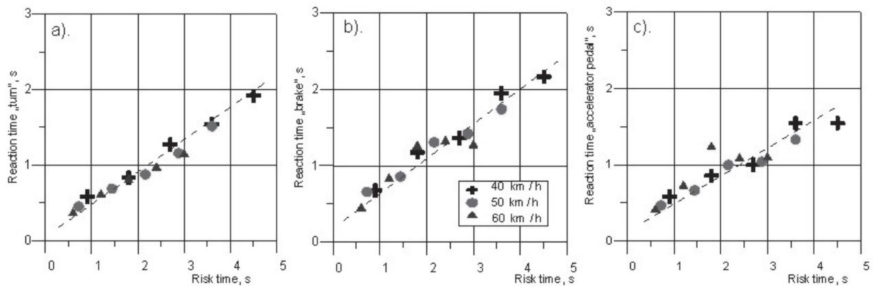
Fig. 6. The reaction time of drivers in the risk time function obtained during testing on the track: a) "turn" reaction time, b) "brake" reaction time, c) "accelerator pedal" reaction time
