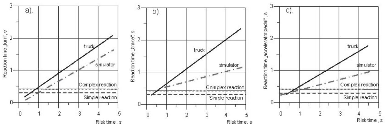
Fig. 10. Comparison of the time for considered manoeuvres: a) “turn” reaction time, b) “brake” reaction time, c) “accelerator pedal” reaction time
