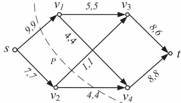
Fig. 5. Optimal network flow
