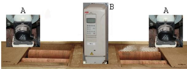
Fig. 1. Roll test bed: A - Incremental sensor of roller's revolution, B - Frequency converter
