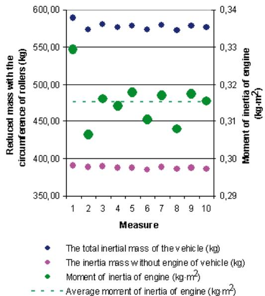
Fig. 3. Results of repeated measurement of inertial mass and moment of inertia of engine
