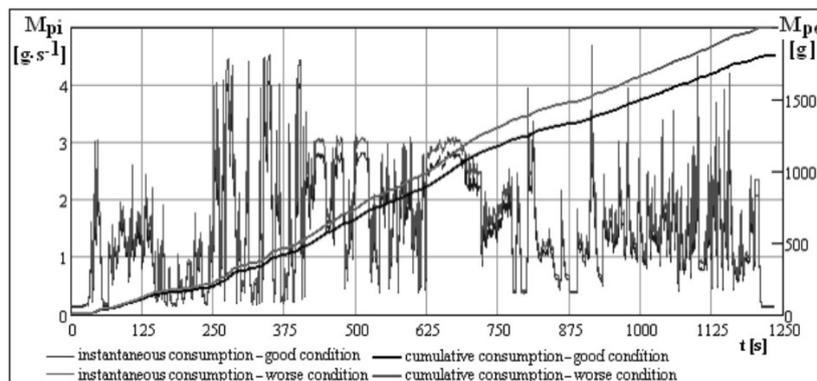
Fig. 2.5. The course of immediate and cumulative fuel consumption in NRTC cycle
