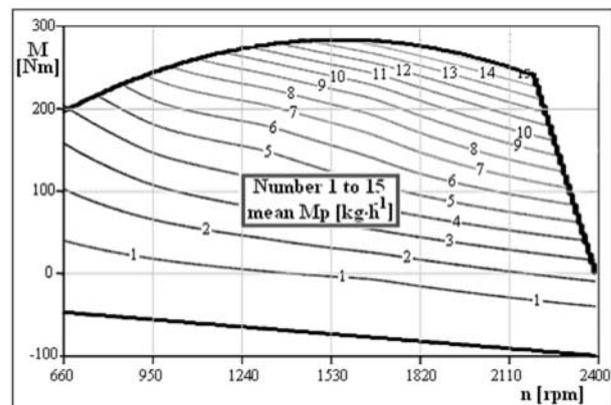
Fig. 2.1. The hourly fuel consumption in dependence of engine speed and engine torque
