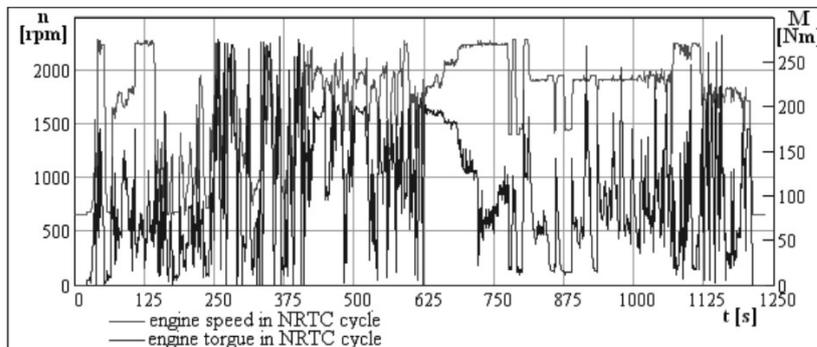
Fig. 2.4. The course of engine speed and engine torque in NRTC cycle
