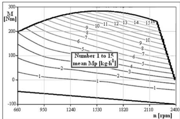
Fig. 2.2. Hourly fuel consumption in dependence of engine speed and engine torque
