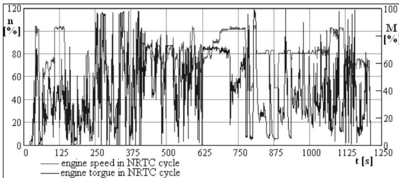
Fig. 2.3. The course of percentage engine speed and engine torque in NRTC cycle
