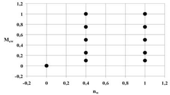
Fig. 2. Type B universal test according to ISO 8178–4 standard
